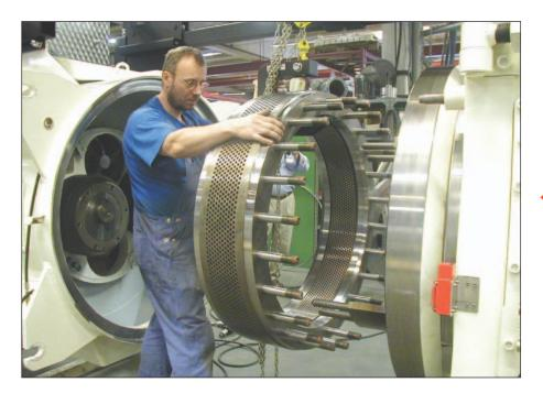
Matrix being set up to press sawdust into pellets. as they will rapidly take up moisture, swell and disintegrate if exposed to water. The truck should always be carefully covered with a water-tight tarpaulin to keep rain out.
