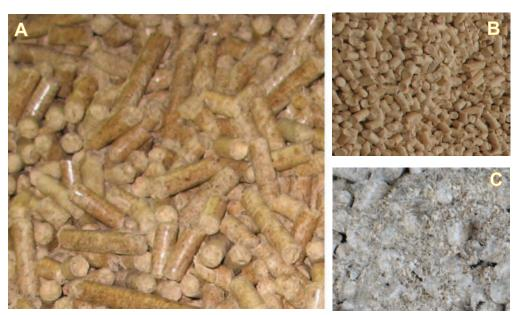
(A) Good quality pellets; (B) medium quality pellets; (C) poor quality pellets.
